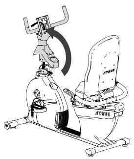
D. Place the front mast onto the bike frame.
