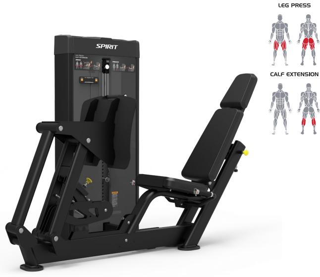
The Leg Press and Calf Extension machine comes equipped with a footplate and adjustable backpad angle which provides ideal positioning for both leg and calf pressing. The four-bar linkage in the footplate allows users to maintain ergonomic ankle alignment throughout each movement, as well as an angled lower section to help with calf press positioning. An integrated rep counter keeps users motivated set after set, while built-in storage on the top cap keeps accessories close by.
