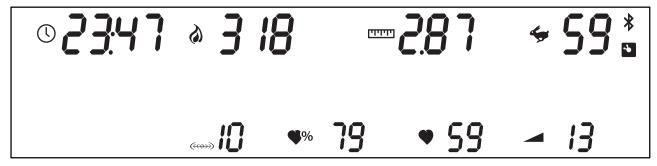
The top portion of the standard console is an LCD which prompts you to enter important information, dynamically displays all of the important workout data, and highlights aspects of your workout such as upcoming intervals and resistance changes. Watch the display as you set up and progress through your workout—it will guide you, motivate you, and reward you with summary information at the end of your session.
