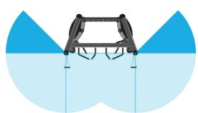
Vertical adjustment columns **rotate 360°** to allow unrestricted movement in multiple planes.
