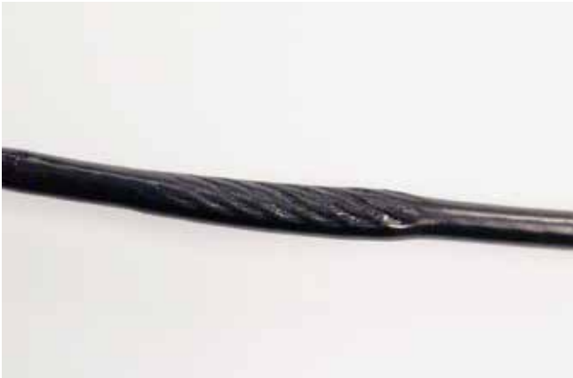
"NECKING", STRETCHED CABLE COVERING
