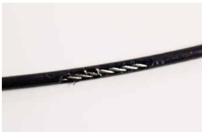
A TEAR IN THE CABLE COVER
