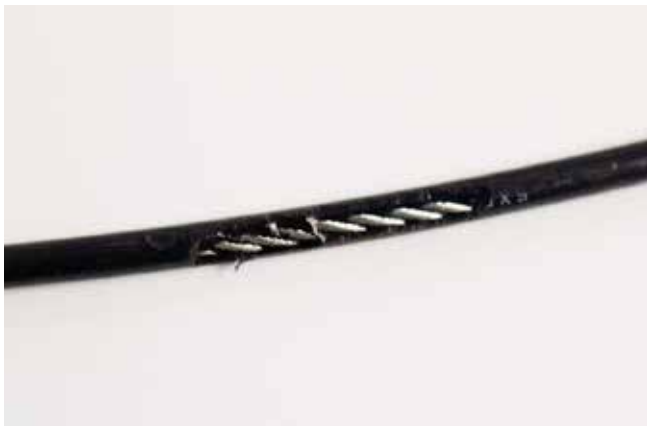
A TEAR IN THE CABLE COVER
