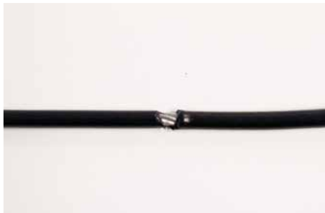
A CRACK IN THE CABLE COVER
