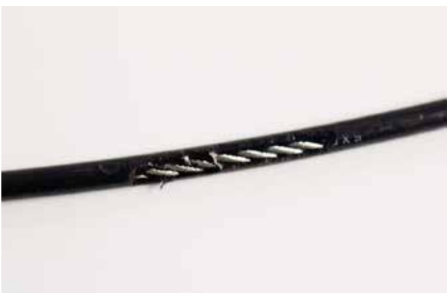
A TEAR IN THE CABLE COVER
