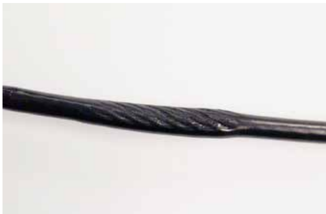
"NECKING", STRETCHED CABLE COVERING
