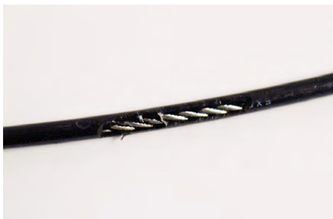
A TEAR IN THE CABLE COVER
