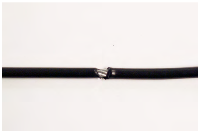
A CRACK IN THE CABLE COVER
