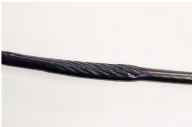
"NECKING", STRECHED CABLE COVERING
