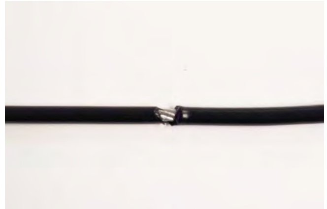
A CRACK IN THE CABLE COVER
