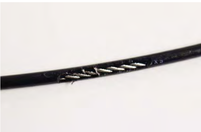
A TEAR IN THE CABLE COVER
