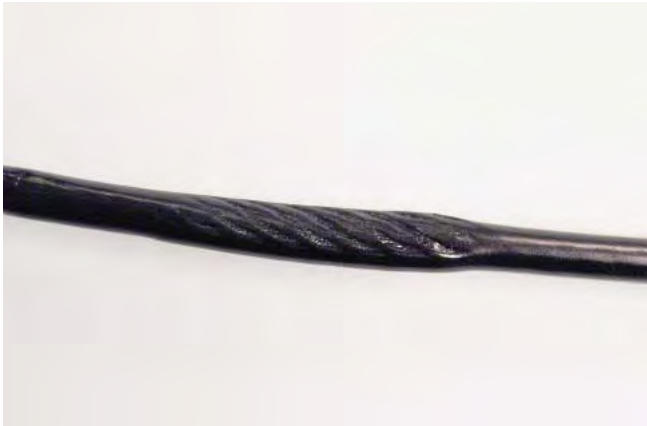
"NECKING", STRECHED CABLE COVERING
