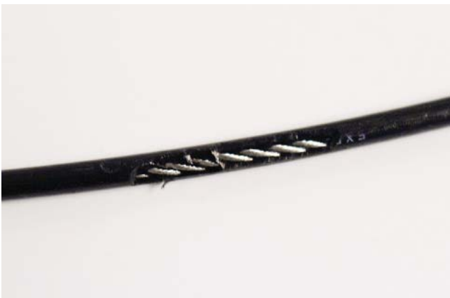
A TEAR IN THE CABLE COVER
