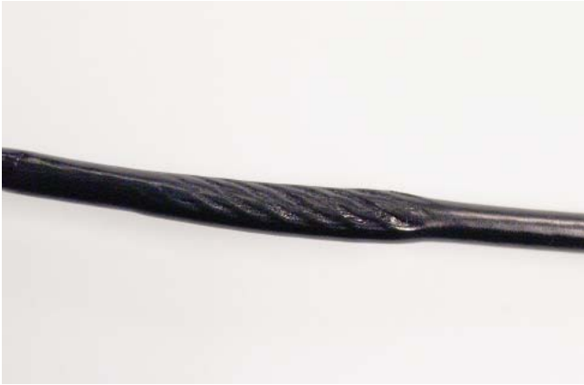
"NECKING", STRECHED CABLE COVERING
