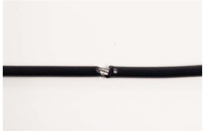
A CRACK IN THE CABLE COVER
