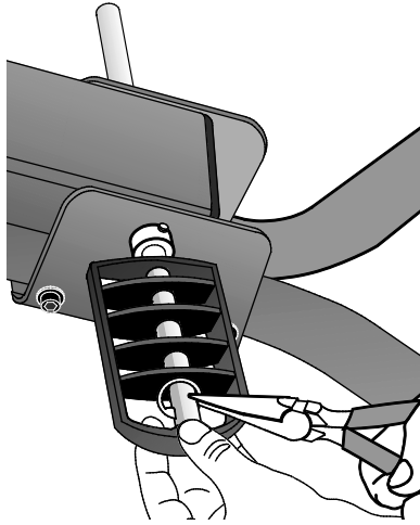
Figure 10: Position of E-clip on the foot rest
