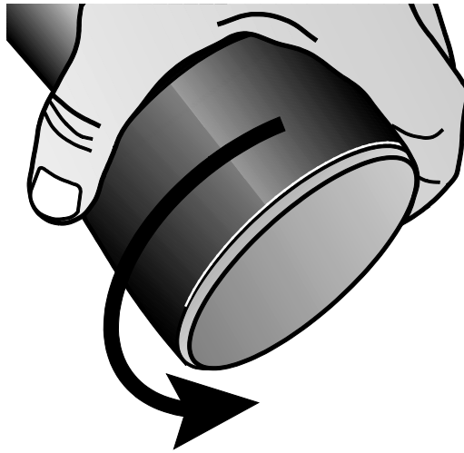
Figure 15: Rear level adjuster
